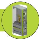
Simple and compact RoboCube automation cell with a footprint of 1,1m<sup>2</sup> and capacity for small extensions. The cell front is open and faces the processing machine. The side walls are adapted to the contour of the processing machine and complete the protected area.
