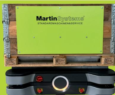
**Function:** Thanks to the electrically powered and ultra-flat pallet short-stroke module, the AMR drives under the pallets and lifts them up.
